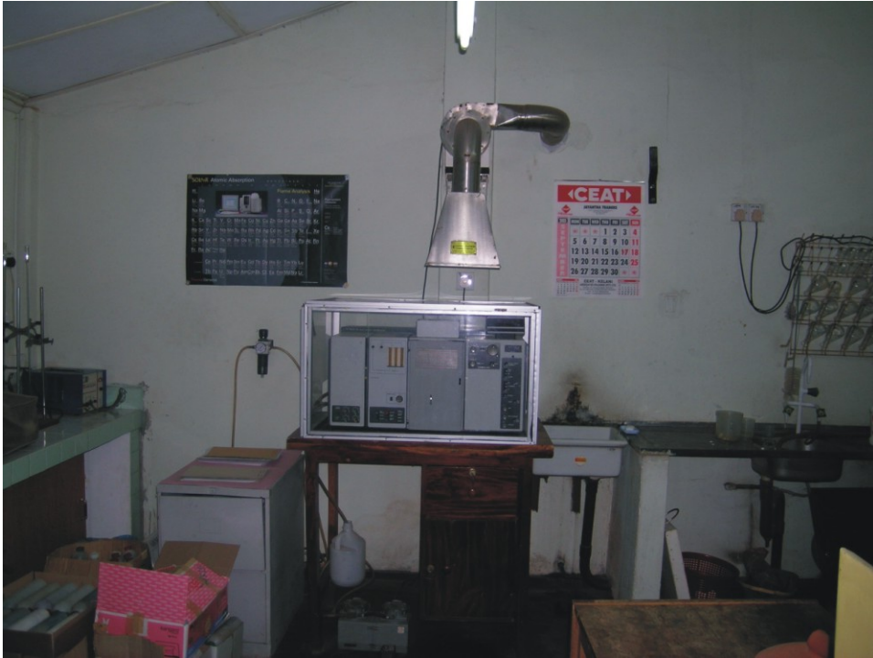
Figure 3. Atomic absorption spectrometer for measuring specific cations. At the water chemistry laboratory of the Water Resources Board in Colombo.
