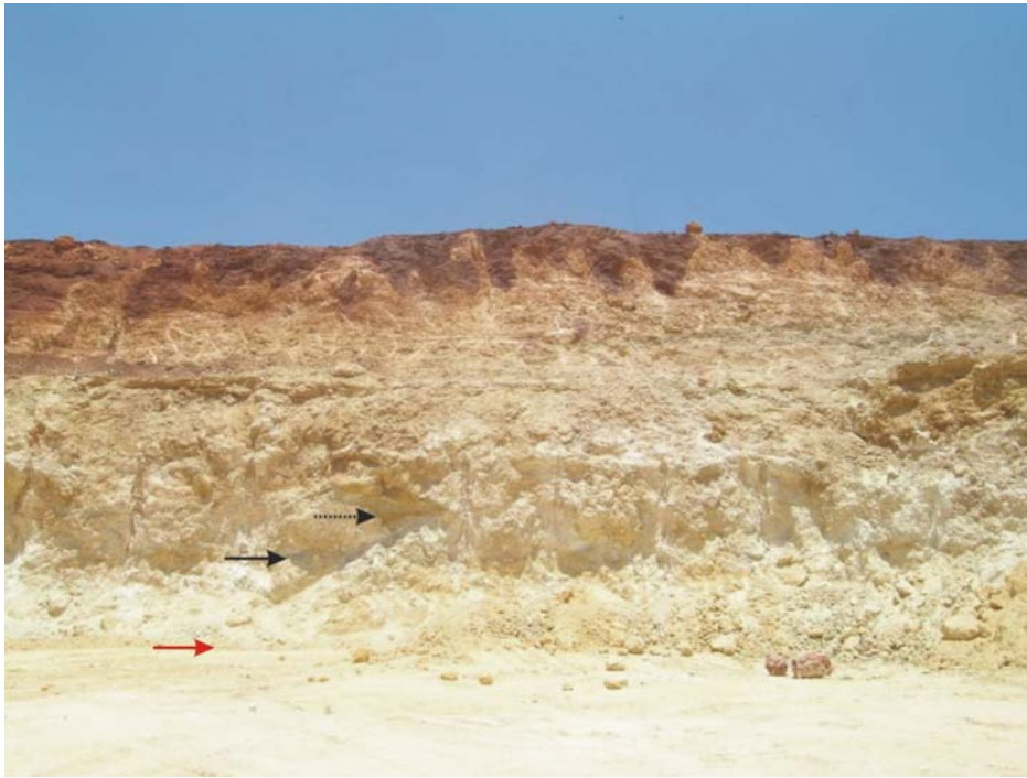
Figure 9. Limestone quarry near village of Aruwakkaru. These limestone rocks are part of the confined Miocene limestone aquifer where present below the water table. The red arrow points to the quarry floor, which corresponds to a geologic contact between sandy clay or sand and clay (per. comm., quarry engineer) that underlies the overlying cream or yellowish colored limestone quarry walls. The lowermost black arrow shows the location of a laminated calcrete that represents a subaerial unconformity. The overlying dashed black arrow may also be a laminated calcrete. The dashed arrow shows about the maximum vertical extent of the quarry wall that was observed at close hand. Visible near the top of the quarry wall is pinnacle karst defining the top of the Miocene limestone that is filled in with maroon Pleistocene siliciclastics of the overlying regional confining unit.
