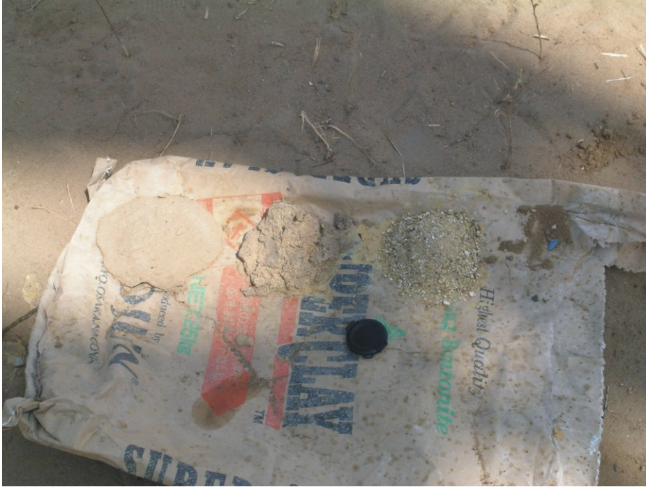
Figure 7. Three sediment samples of the shallow confining unit collected from the subsurface at the drill rig near prawn farm at Karadipual.
