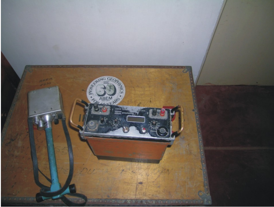
Figure 11. Resistivity instrumentation that has been used by the Kalladi Water Resources Board office during water resource exploration activities.
